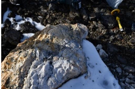
Figure 4-1: A 2 cm deep grid was cut into the boulder using an angle grinder (a). Cubes of rock were then removed from the boulder using a chisel and hammer
