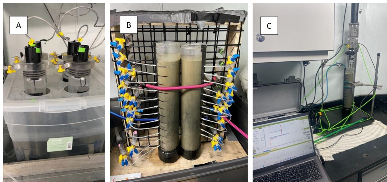
Figure 39-4: Flux incubation experiment setup demonstrating capped cores with spinning motors in a cool water bath (A). Porewater being extracted by rhizons and syringes every \sim 2 cm down the cores (B). Micro-profiling oxygen with our microsensor (C) with an example of the plot it generates. The horizontal spikes in oxygen on the plot occurred when the bow thruster was being used and the counters were shaking.
