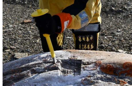
Figure 4-1: A 2 cm deep grid was cut into the boulder using an angle grinder (a). Cubes of rock were then removed from the boulder using a chisel and hammer
