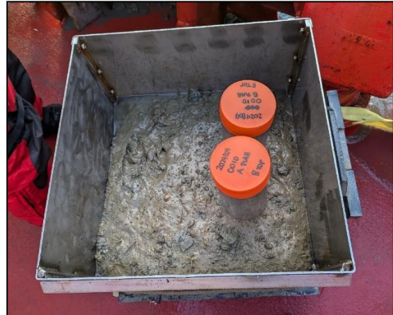
Figure 47-7: Example of push core subsampling from NRCan box core station 0010.
