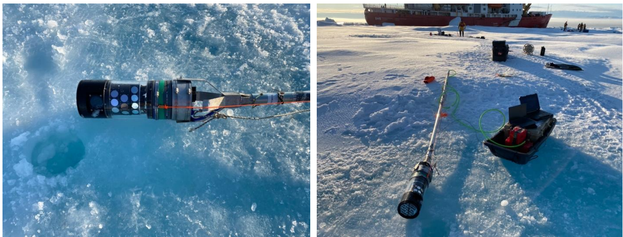
Figure 9-3: Lidar setup prior to measurements under ice.
