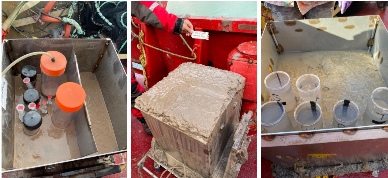
Figure 39-3: Photos of a boxcores sampled from A) Maqtaq Fjord, B) Coronation Fjord and C) North Pang Fjord with overlaying water drained but still in core tubes (Leg 2b)
