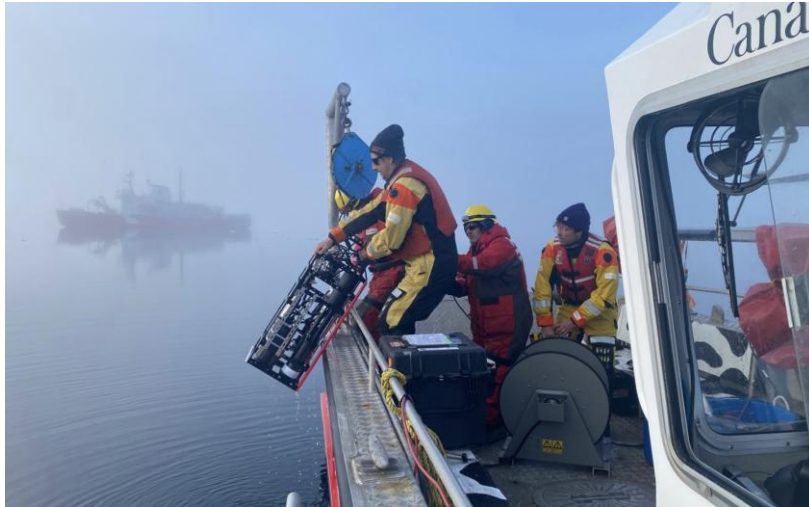
Figure 9-4: Optical frame deployment from the barge
