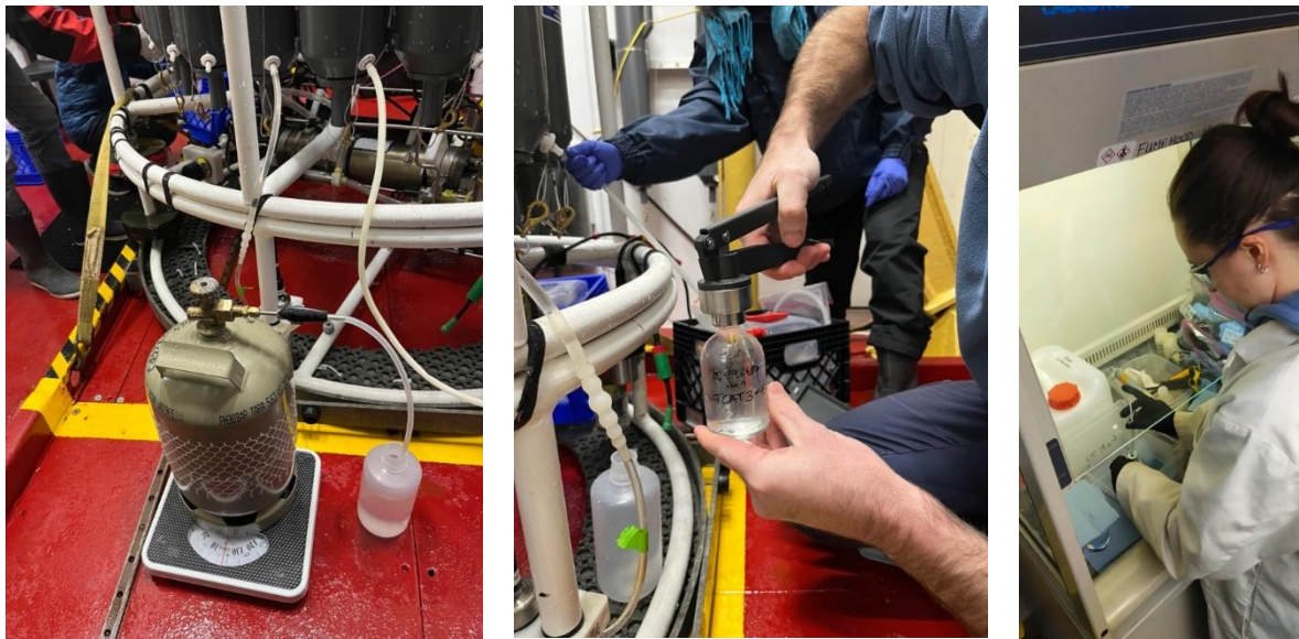
Figure 12-1: Sampling for ^{39}\text{Ar} samples, ^{14}\text{C} , and poisoning ^{14}\text{C} samples with mercury chloride
