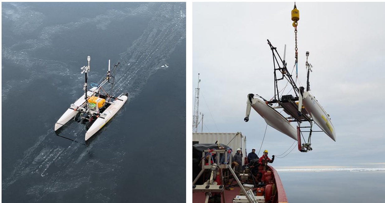
Figure 5-6: The Flux Catorator. Left panel is the FC displaying icebreaking capabilities in thin nilas ice. Right panel is deployment by crane from Amundsen starboard bow. The Flux Catorator was deployed and recovered from the deck of the vessel using a crane. It was capable of approaching and leaving the vessel under remote control and performing autonomous missions.
