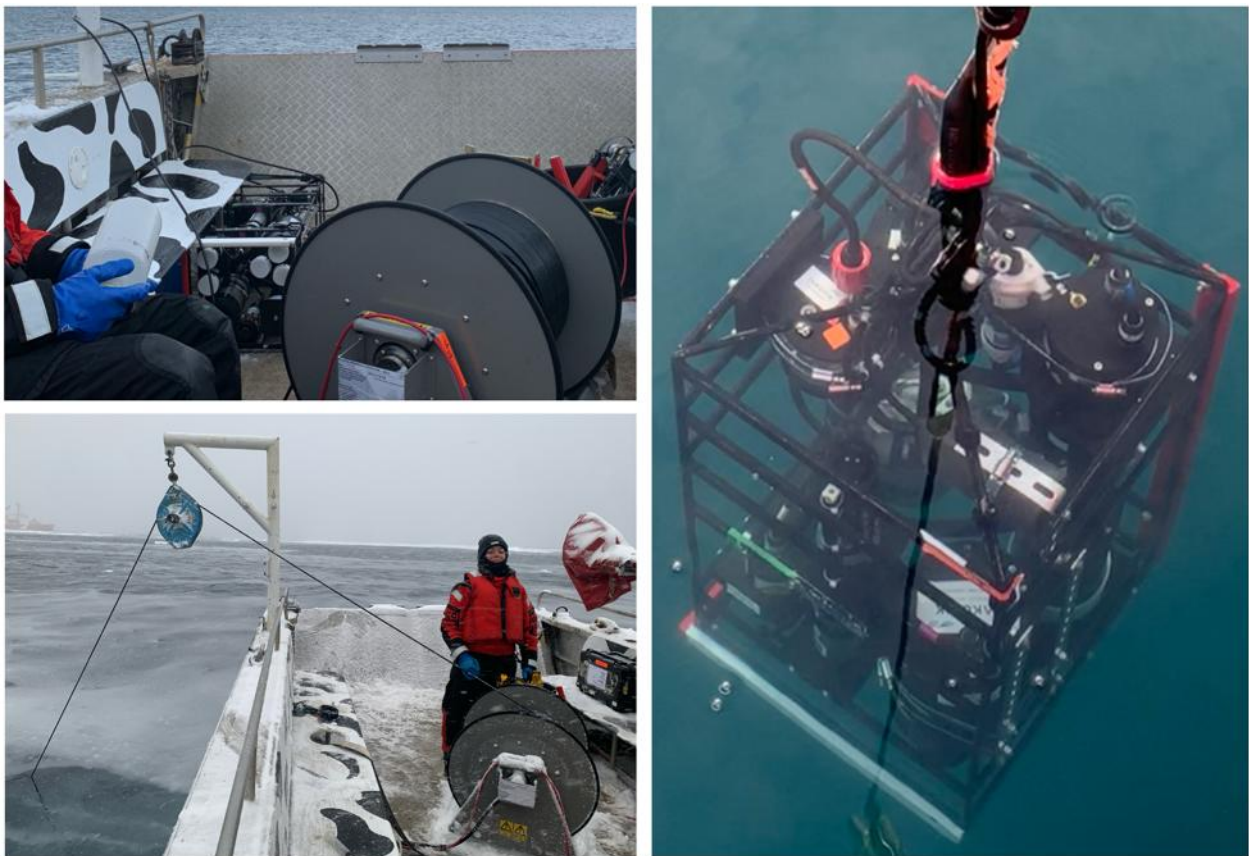
Figure 8-2: Top left: The IOP frame is lying flat on the barge deck, next to the winch. Bottom left: The IOP frame is lowered at sea using the drill-operated winch and the port side davit. Right: The IOP frame is warming-up/flushing its tubing system system just under the sea surface (after an initial descent for de-bubbling).
