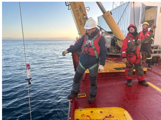
Figure 51-5: An RBR concerto CT logger emerges from the sea during the M2 mooring recovery operation.
