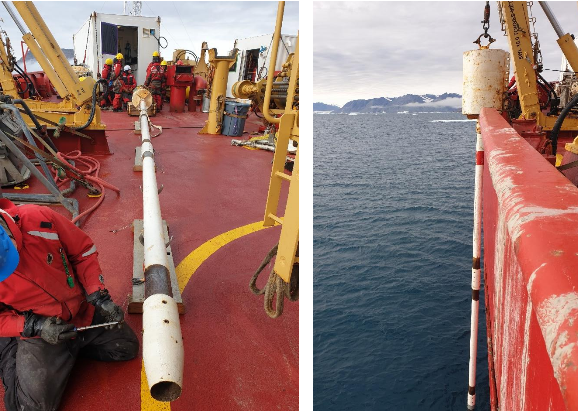
Figure 48-3: Assembly of the giant gravity core three barrels (left) and deployment of the giant gravity core two barrels (right) (Elodie Bracquart)
