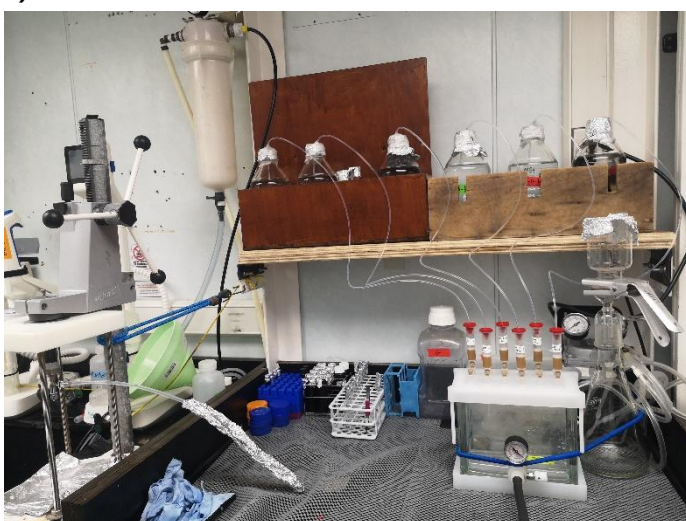
Figure 30-1: a. The rosette coming out of the water, b. filtration system in the aft lab on board the Amundsen, and c. chemistry bench to process samples for DOM, FDOM, DOC and aa analysis.
