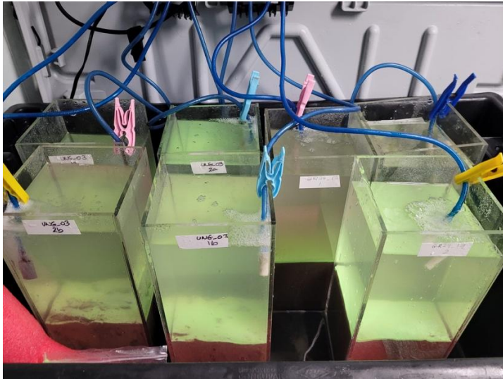
Figure 46-1: Set-up of the experimental aquaria containing intact infaunal benthic communities from three stations in Ungava Bay, Canada. All aquaria were continually aerated and maintained for 5 days at 4°C in the dark. Green layer on the sediment surface is dyed sand used for the quantification of sediment reworking (bioturbation) by the infaunal community.
