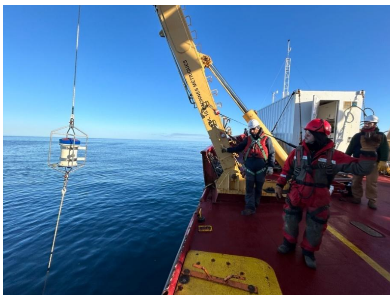
Figure 51-6: A 300 kHz Workhorse ADCP by Teledyne RDI is recovered on mooring M3. It was deployed for over a one year at about 80 m depth and had very little biofouling.
