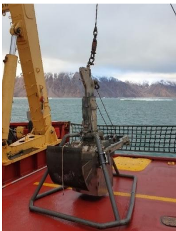
Figure 48-1: Deployment of the box corer (photo: Elodie Bracquart)
