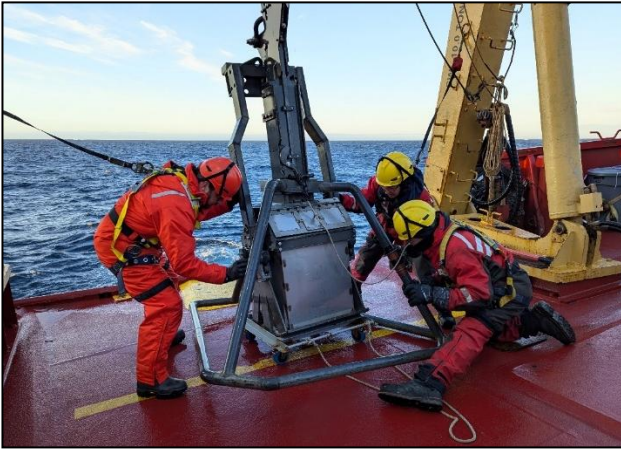
Figure 47-6: Deployment of the box core system.
