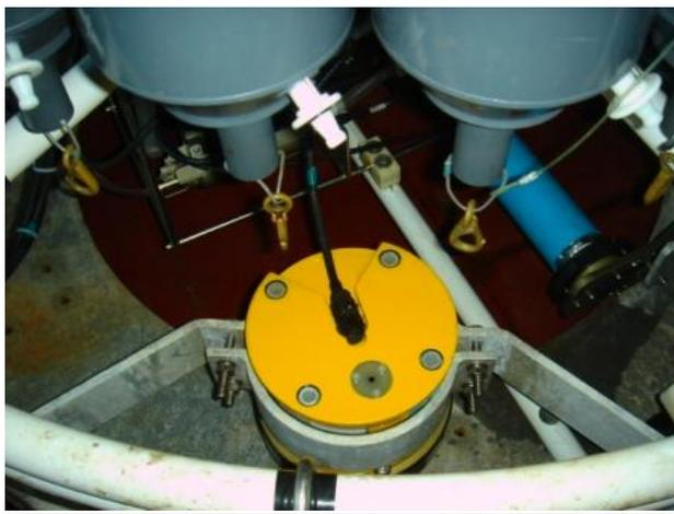
Figure 10.20. RDI LADCP mounted on the bottom of the SBE32 carousel on the *Amundsen*.
