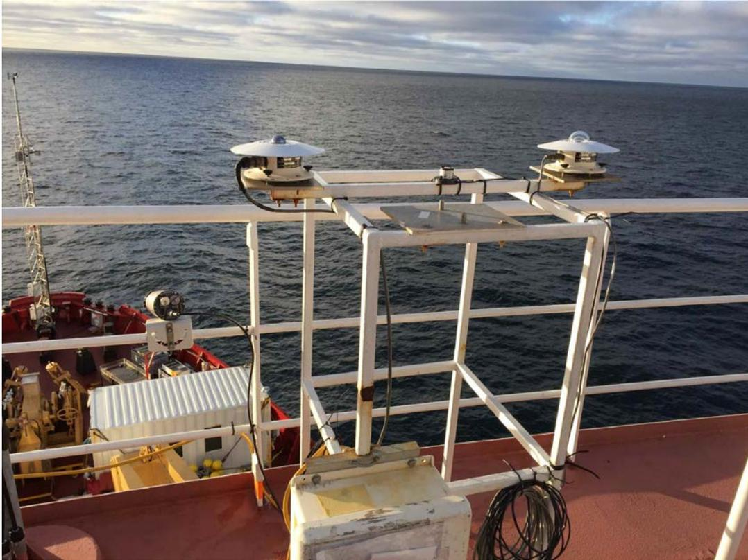
Figure 2.1. The radiation sensors and digital camera located above the wheelhouse of the Amundsen. Shown are the pyrometer (left), pyranometer (right) and PAR sensor (centre). The automated digital camera is mounted on the rail below and to the left of the pyrometer.
