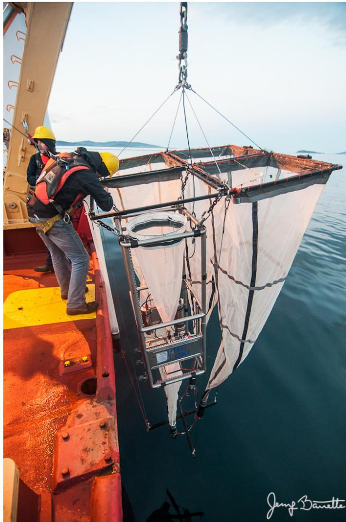
Figure 28.2. The 5-net vertical zooplankton sampler with LOKI (Monster net). (photo: Jessy Barrette 2013 ArcticNet Leg 1a)
