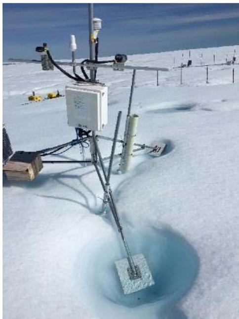
Figure 3.1. Weather station and ablation stakes on Ice Island PII-2012-A\_1-f, July 27, 2016. Photo courtesy of Luke Copland.
