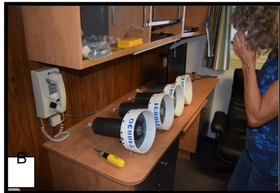
Figure 9.8 Sediment trap timers All timers were set simultaneously and turned on at the exact same time at 0:00 Hr on 4-October-2016.
