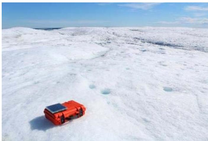
Figure 3.3. Example of placement of RockStar beacon on ice island. Deployed SE of Sam Ford Fiord, July 31, 2016. Photo courtesy of Abby Dalton.
