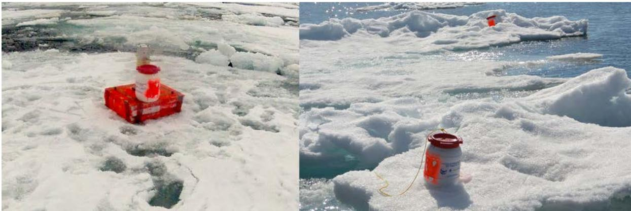
Figure 4.2. Deployment of the Aquadopp on an ice floe, within the MIZ (left panel), and the wave buoys alone (right panel).
