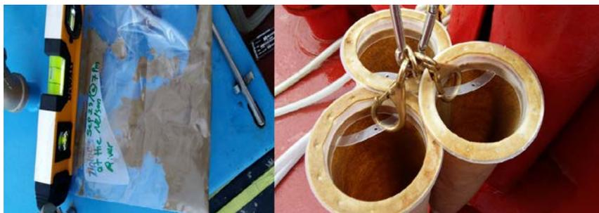
Figure 9.27 Industrial centrifuge set up, suspended sediment samples, and collection tubes
