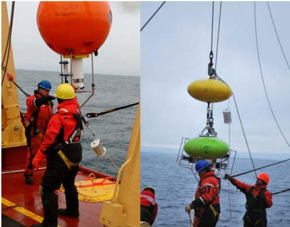
Figure 28.1. SPMD cage installed on the mooring line on BREA mooring BR-3 (left) and BR-K (right).
