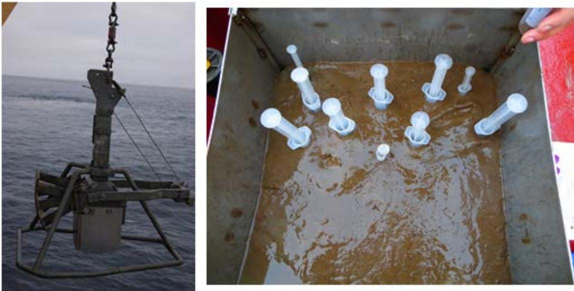
Figure 32.1. *Box core deployment and sediment cores sampling.*
