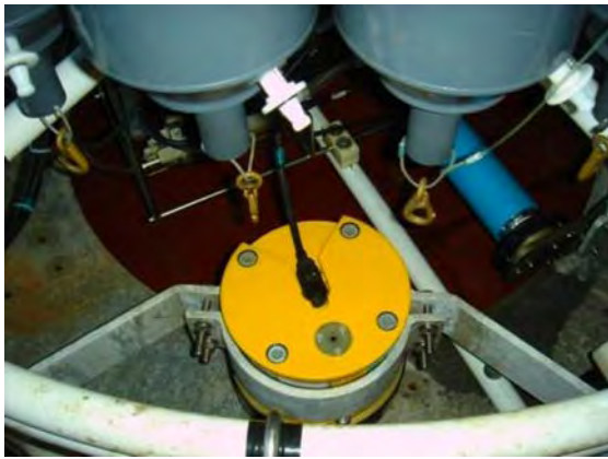
Figure 9-7. RDI LADCP mounted on the bottom of the SBE32 carousel on the Amundsen .
