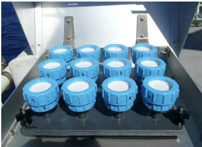
Figure 3-1. The PVC adapter plate that holds 12 – 47mm filter holders (courtesy of Bill Landing).
