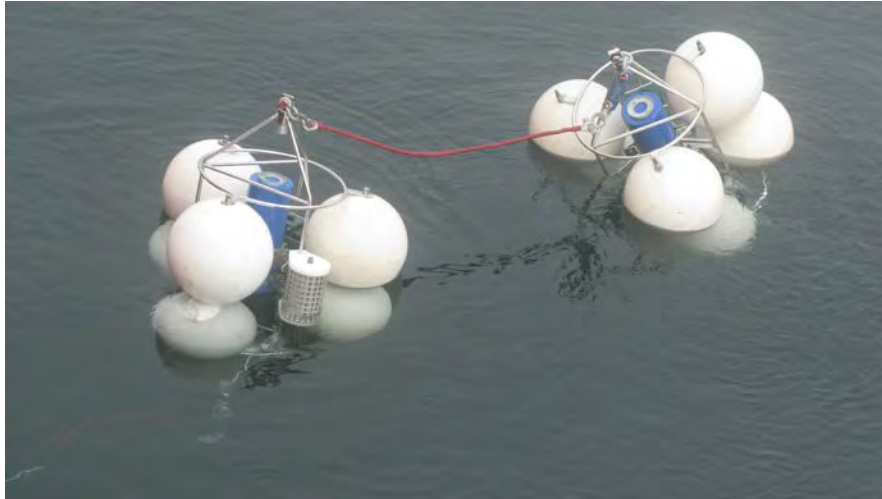
Figure 31-3. SPMD cage installed on ArcticNet mooring BS-3.
