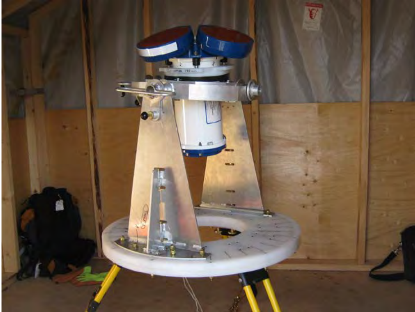
Figure 8-3. Tilt and rotate calibration jig / table as utilized in Inuvik, NWT
