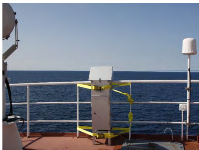
Figure 3-3. The TISCH volume flow controlled (VFC) high volume aerosol sampler deployed on the bridge deck of the CCGS Amundsen during Leg 3b from September – October, 2015 (left). The anemometer, which is attached to the aerosol sampler through CR10 datalogger (right).
