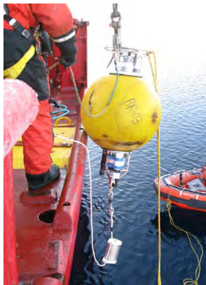
Figure 31-4. SPMD cage installed on the line on BREA mooring BR-3.
