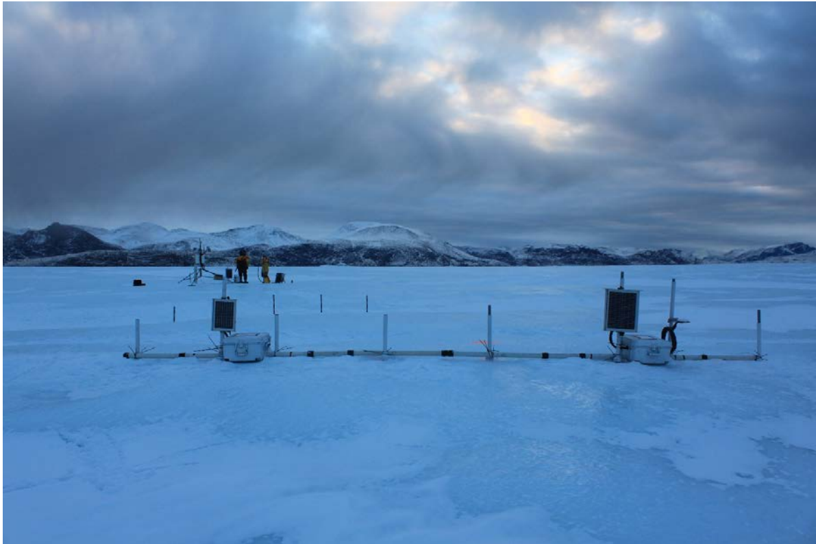
Figure 6-2. Ice penetrating radar (foreground), meteorological station (background) and row of ablation stakes between.
