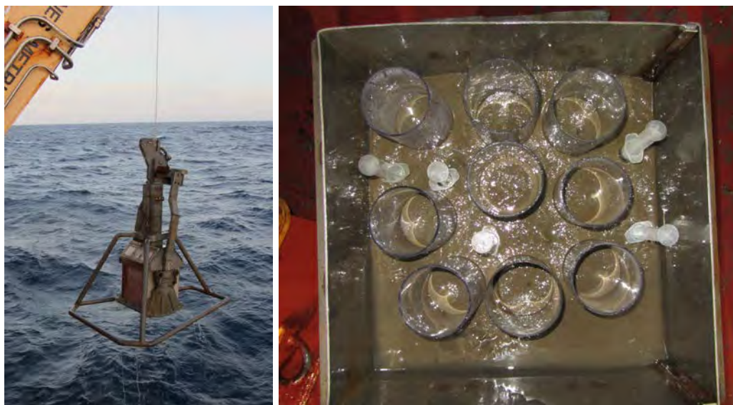
Figure 36-1. Box core deployment and sediment cores sampling.
