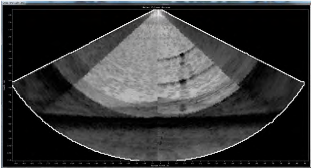
Figure 8-7. Multibeam imagery identifying orientation and instrument depths (screenshot courtesy of ArcticNet multibeam processing team).
