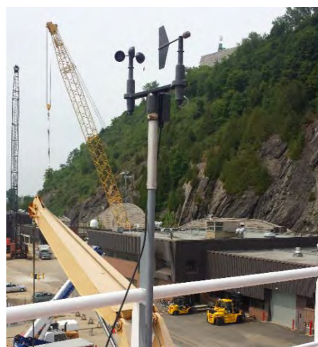
Figure 3-3. The TISCH volume flow controlled (VFC) high volume aerosol sampler deployed on the bridge deck of the CCGS Amundsen during Leg 3b from September – October, 2015 (left). The anemometer, which is attached to the aerosol sampler through CR10 datalogger (right).
