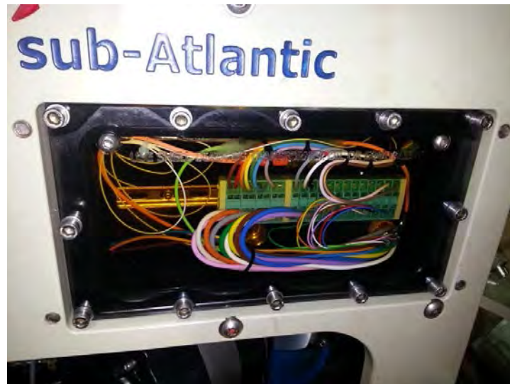
Figure 18.2. The termination Can Post Reterm of the ROV.
