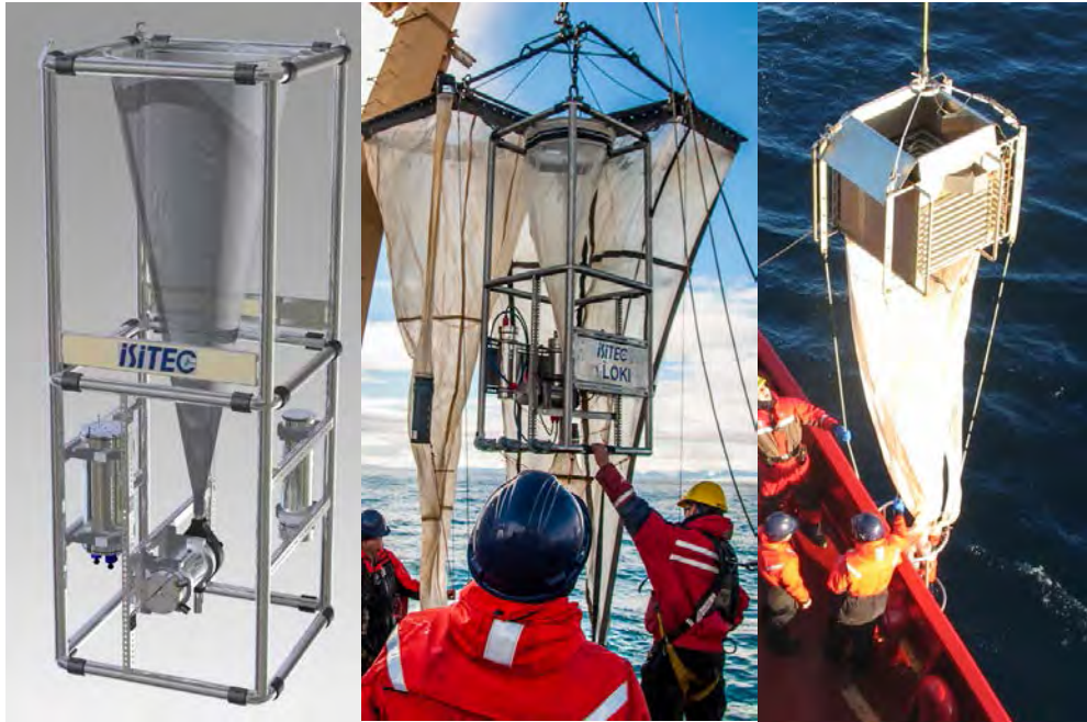
Figure 13.1. Vertically towed equipment used to sample zooplankton. Left: Schematic of LOKI, Middle: 5NVS with the LOKI as deployed during Leg 1 (Photo J. Barette), Right: Hydrobios being deployed (Photo S. Prinsenbergl).
