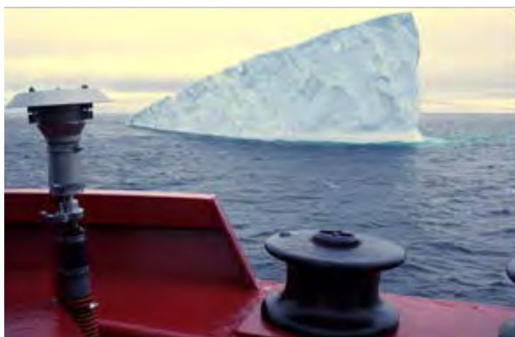
Figure 15.1. Passive air sampler, located at bow of ship, used to collect air samples for contaminants analyses.
