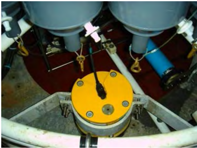
Figure 5.6. The LADCP equipped on the Rosette frame to measure current velocities in the water column.
