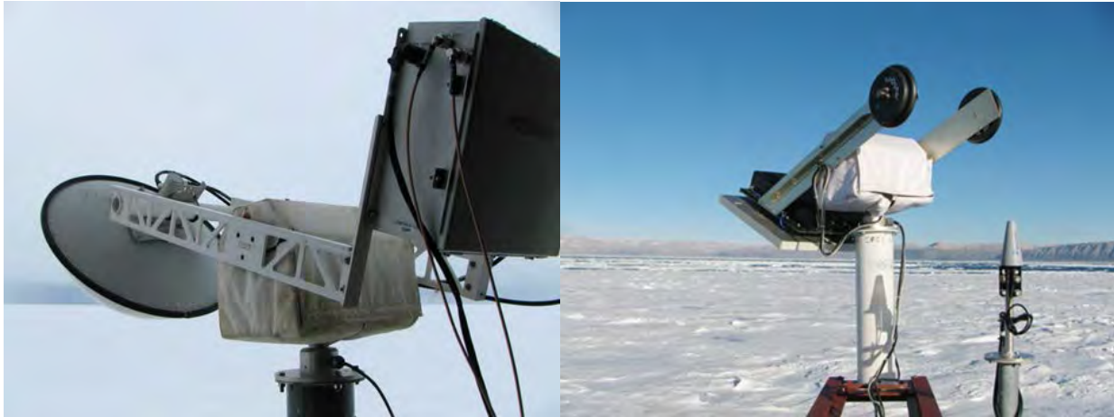
Figure 2.1. Left: C-band scatterometer system mounted on the port side of the ship. Right: L-band scatterometer system.
