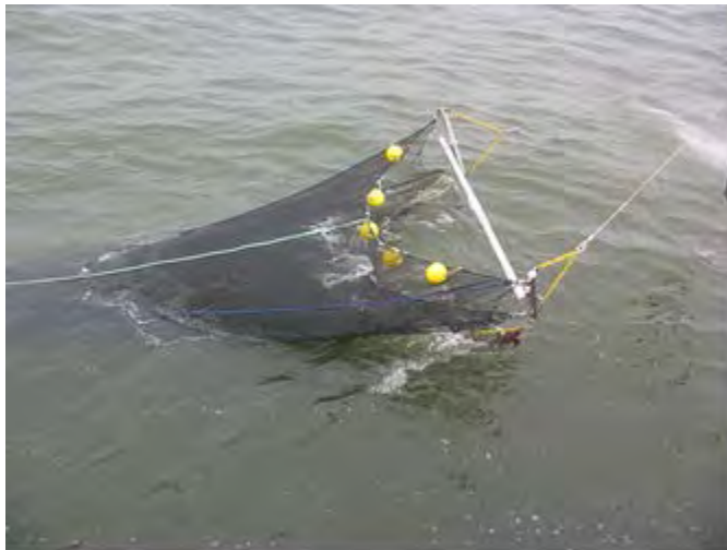
Figure 13.3. The benthic beam trawl used to collect demersal fish (Photo: DFO Winnipeg).
