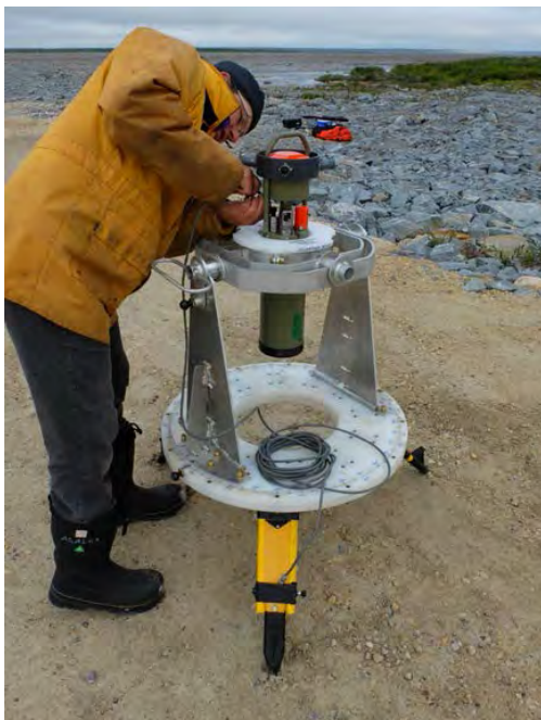
Figure 4.4. The calibration table / jig leveled and loaded with an RCM 11 being readied for calibration before deployment on the mooring.
