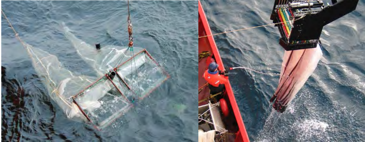
Figure 13.2. Obliquely towed sampling gear to capture fish larvae. Left: DNS at the surface, Right: Bioness being rinsed and recovered (Photo S. Prinsenbergl).
