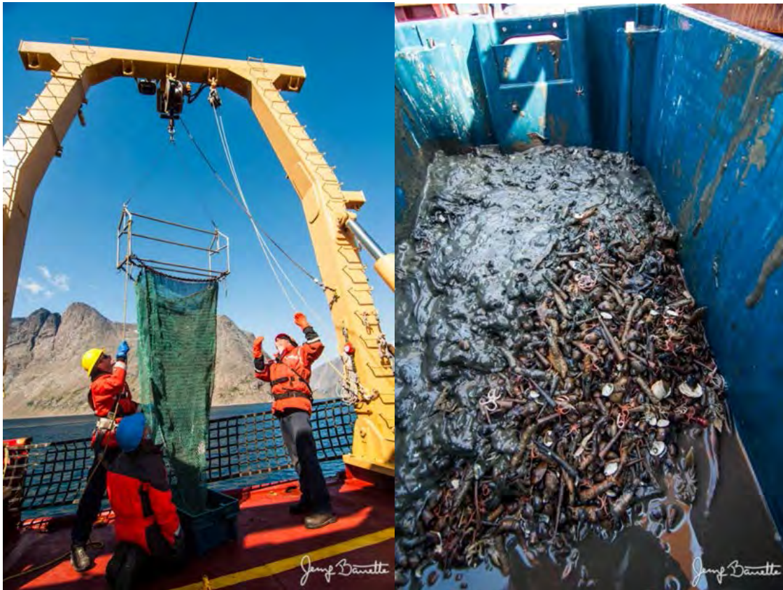
Figure 20.3. Agassiz trawl deployment to collect benthic organisms.
