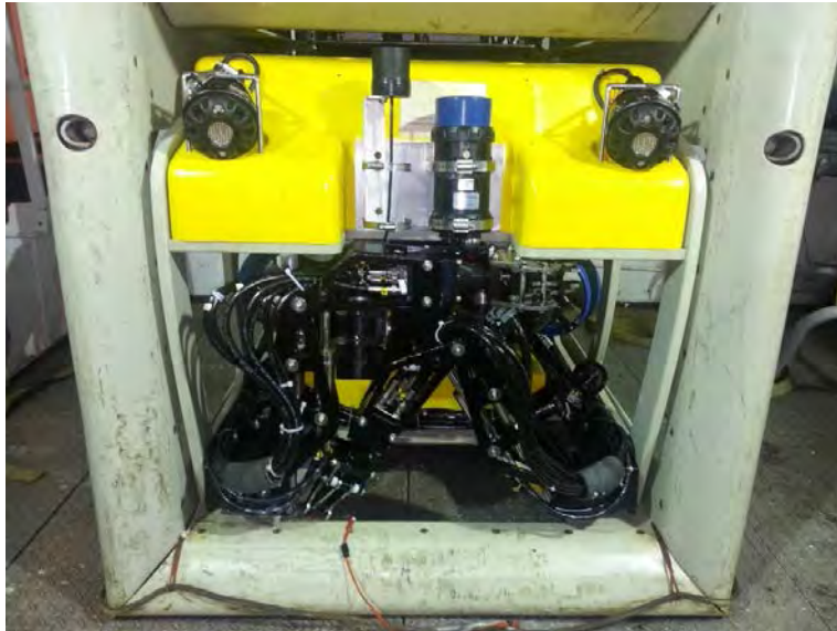
Figure 18.6. The required arm position for recovery of the ROV.
