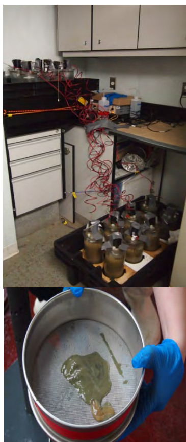
Figure 20.2. Isotope tracing experiment set-up in the temperature controlled room and sieving of sediment samples after finishing the experiment.
