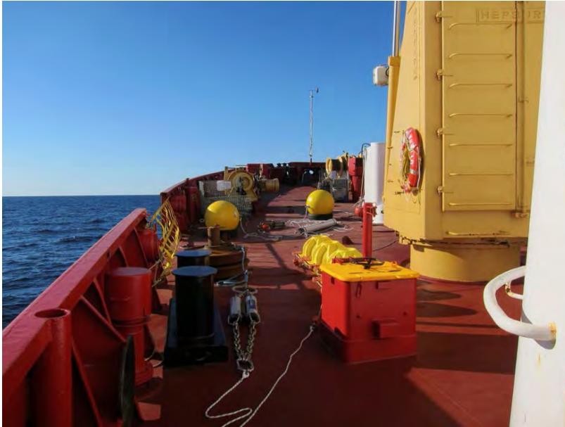
Figure 4.6. Mooring AN01-13 assembled on the foredeck of CCGS Pierre Radisson in Hudson Bay, ready for deployment.
