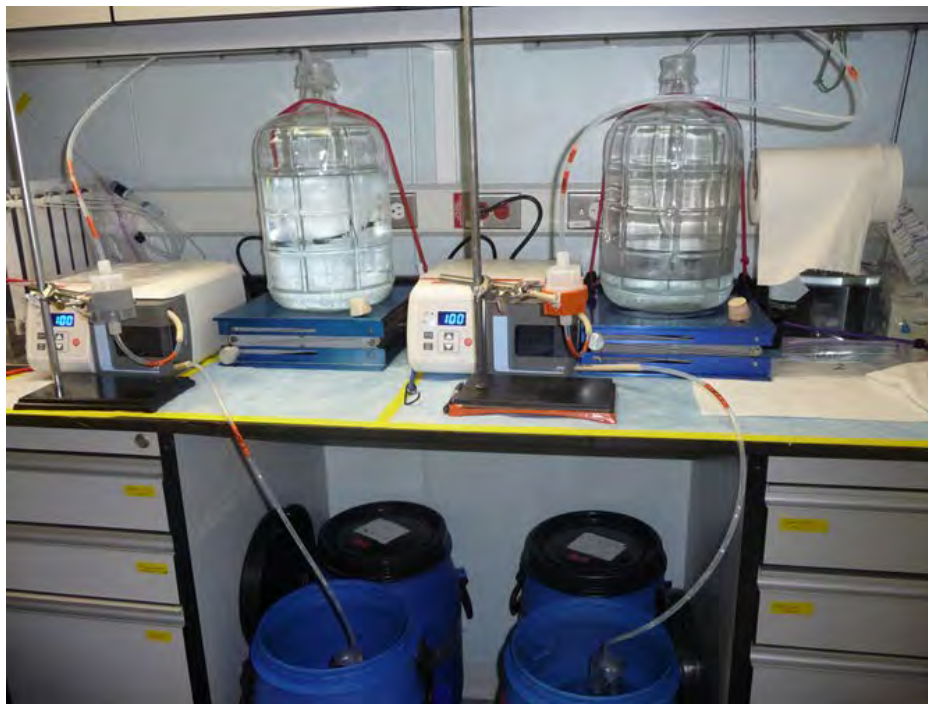
Figure 16.1. Set up for the pre-concentration of mercury from seawater (filtration step).
