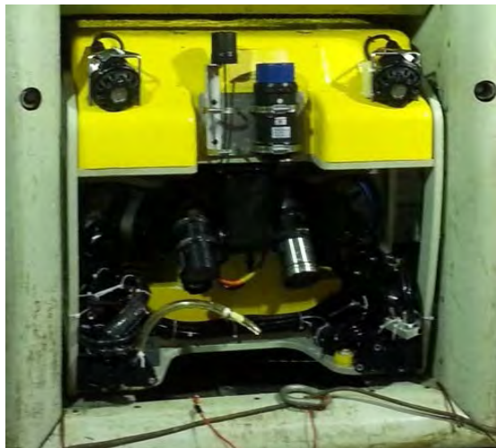
Figure 18.3. The ROV with the arms removed. Note the small white CTD probe inside the transparent hose.
