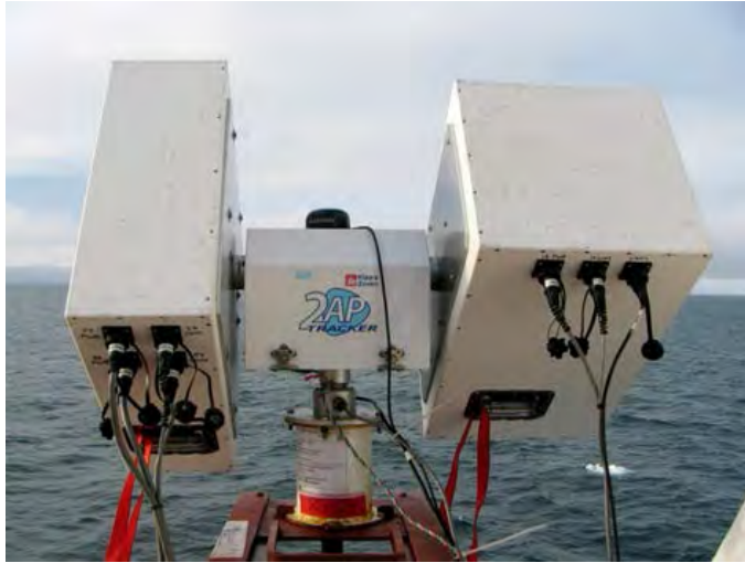
Figure 2.2. Passive microwave radiometer systems.
