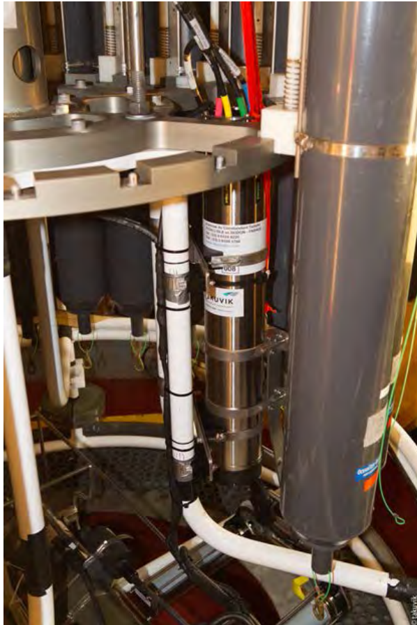
Figure 5.8. The UVP equipped on the Rosette frame to take pictures of particles and organisms in the water column.
