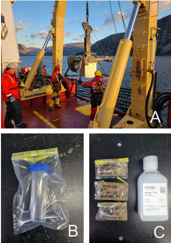
Figure 21-1: Overview of sampling protocol for detection of macroalgae eDNA in marine sediments. A) Deployment of boxcore in Saglek Fjord, B) Sterile mini-core adapted from falcon tube in sterile Whirl-Pak® prior to sampling, C) Three replicate sediments samples preserved with RNAlater™ solution
