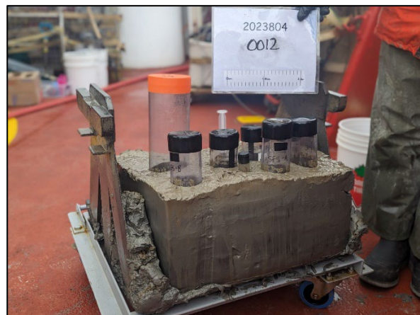
Figure 31-6: Example of push core subsampling from box core station 0012
