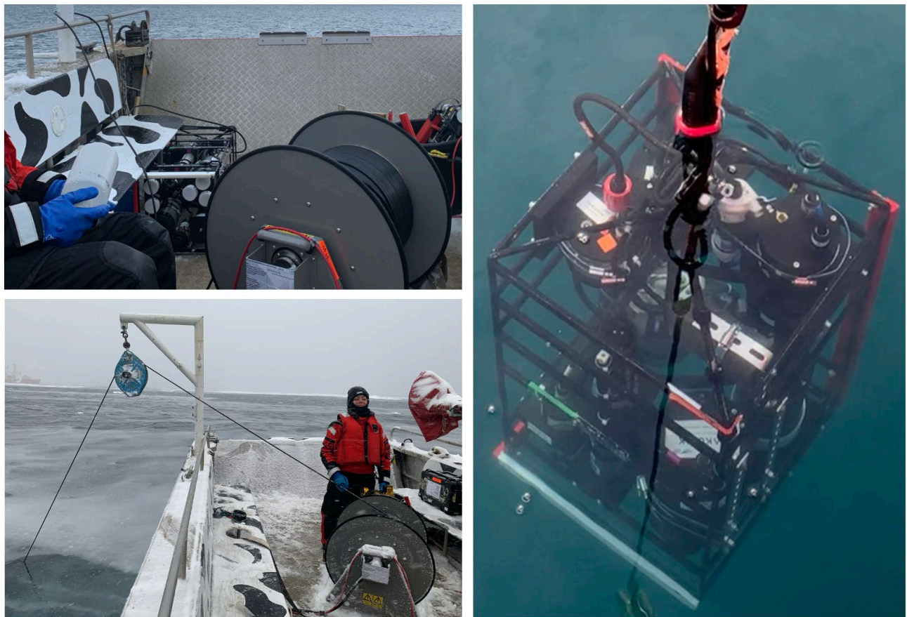
Figure 5-3: Top left: The IOP frame is lying flat on the barge deck, next to the winch. Bottom left: The IOP frame is lowered at sea using the drill-operated winch and the port side davit. Right: The IOP frame is warming-up/flushing its tubing system just under the sea surface (after an initial descent for de-bubbling).
