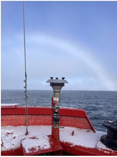
Figure 11-6: Air head set up for OCPs/CUPs/FRs/PFACs/PACs analysis. Photo credit: Haritha Yespal Subha, 2023
