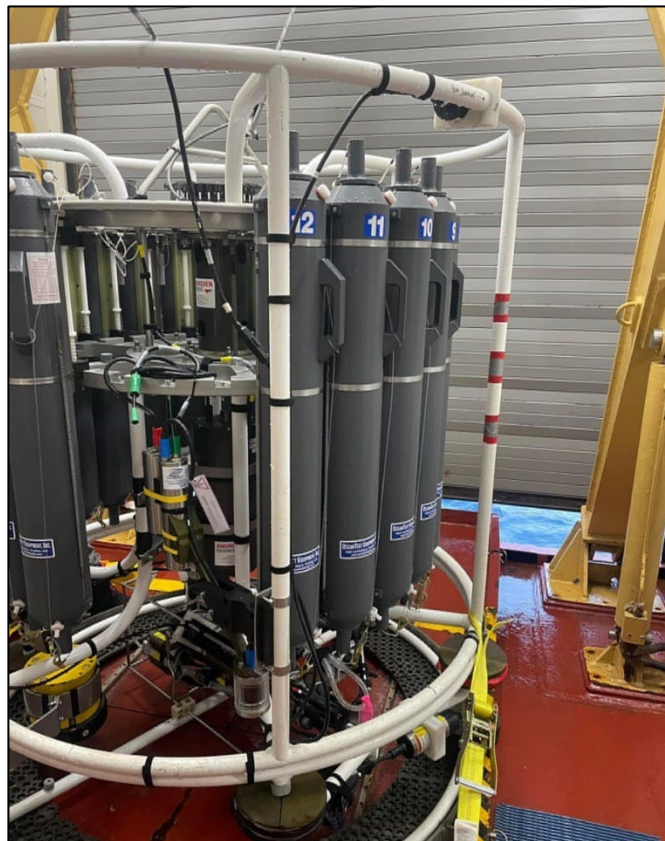
Figure 18-2: UVP-HF6 mounted to the 24 bottle Rosette frame
