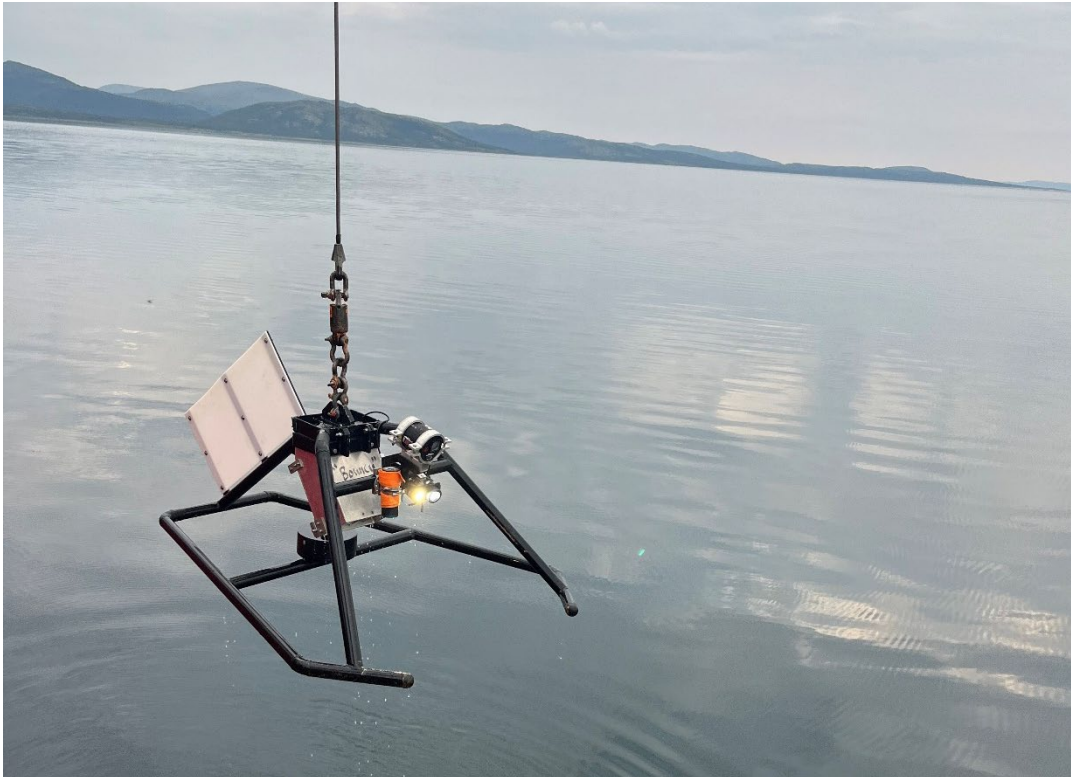
Figure 26-1: The drop camera system attached to a modified box-core frame utilized in Leg 1 of the 2023 Amundsen Expedition
