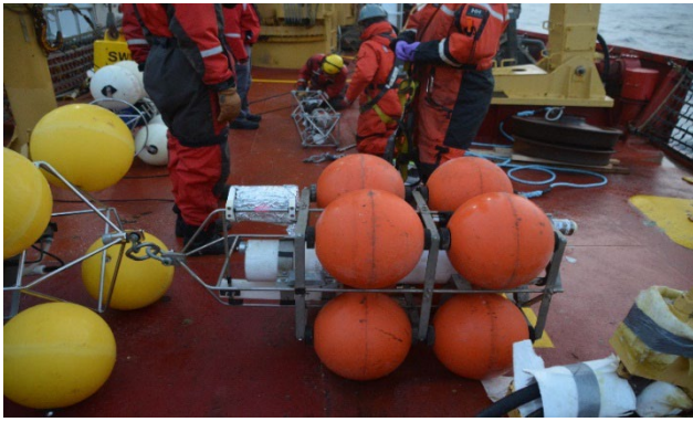
Figure 11-9: Passive sampler deploy at 350 station. Photo credit: Alejandra Granados Galvan, 2023
