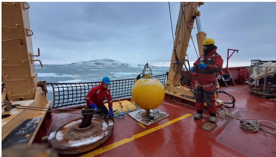
Figure 36-4: Preparing to deploy WBAT-23 mooring in Smith Sound (photo by Emma Ausen)
