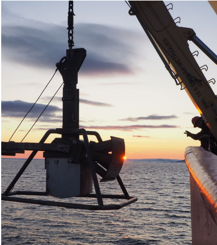
Figure 32-1: Deployment of the box corer (photo: Camille Brice)
