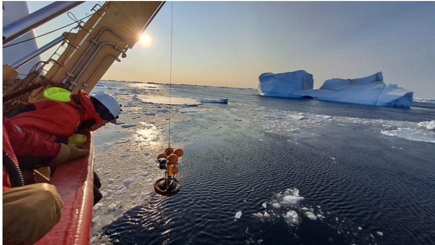
Figure 36-3: Deployment of the M4-CEOS mooring equipped with the auto-release device (photo Emma Ausen).
