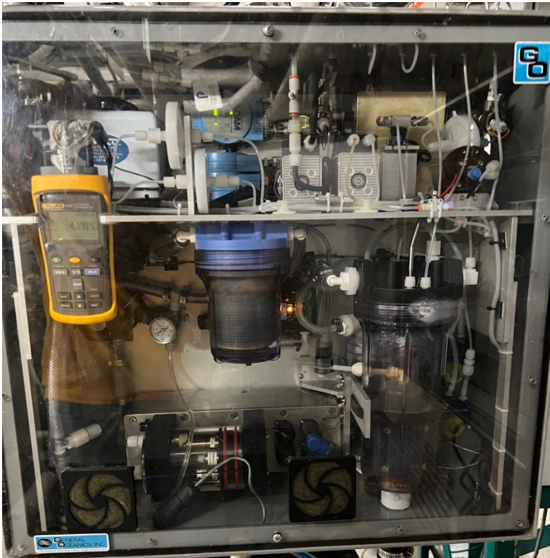
Figure 4-1: General Oceanics 8050 pCO 2 system
