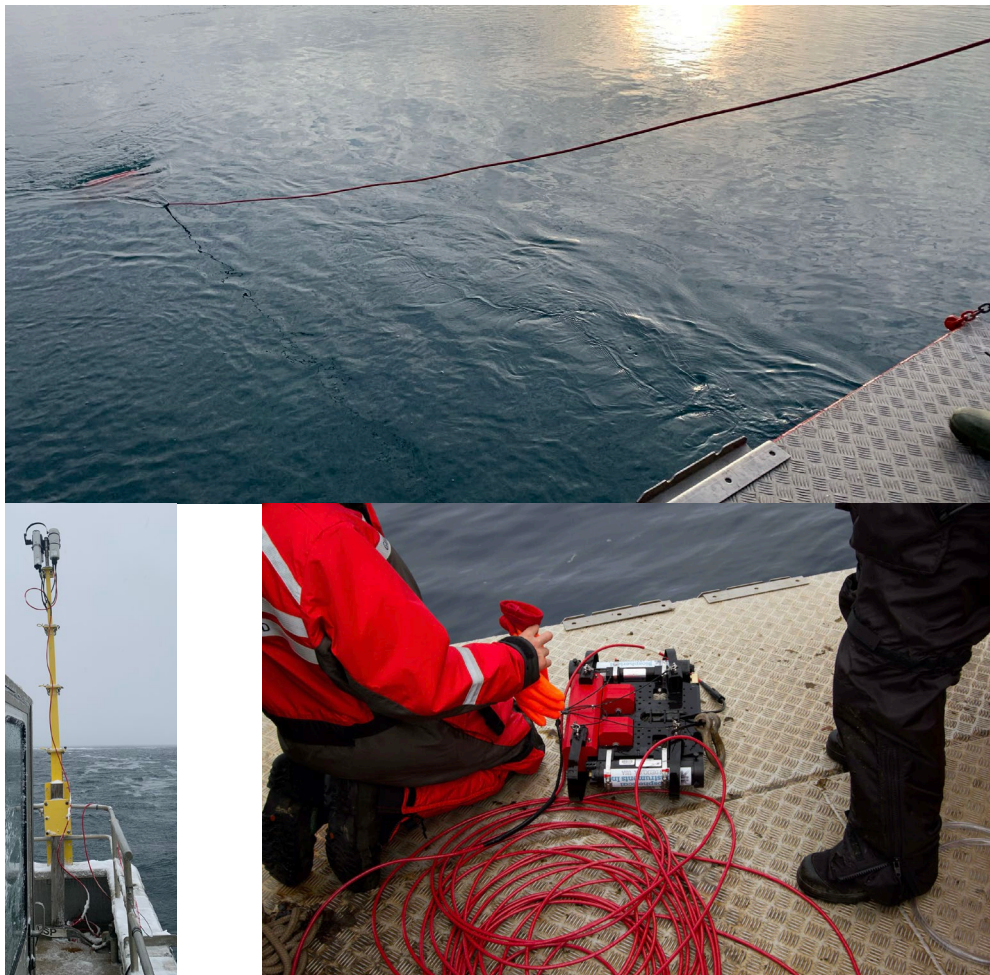
Figure 5-1: Top: The C-OPS is being deployed from the barge. Bottom left: The GPS/shadow band/ E_d0^+ reference on the telescopic mast. Bottom right: The C-OPS after its recovery.
