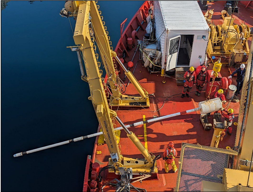
Figure 31-2: Gravity coring system ready for deployment onboard the CCGS Amundsen
