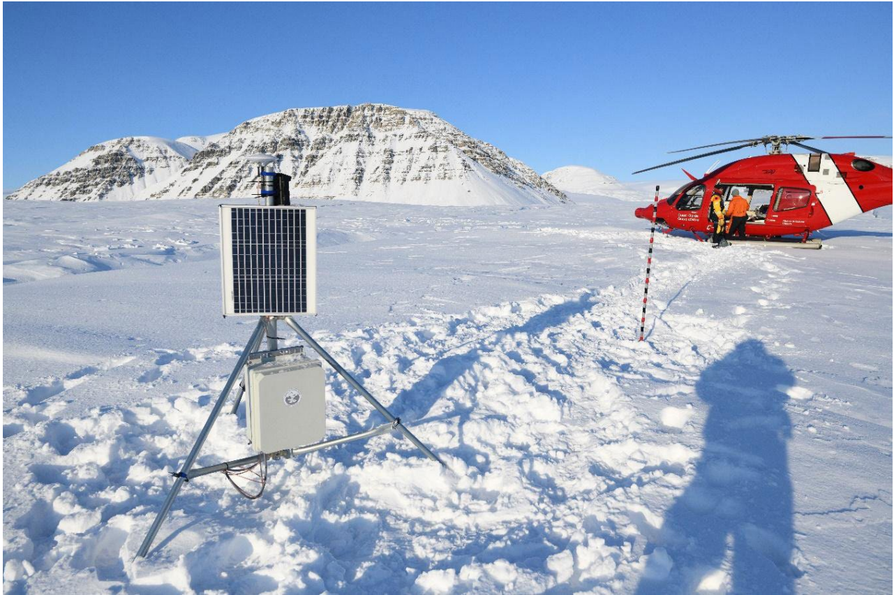
Figure 19-5: Example of the upper glacier velocity tracking system and ablation stake installed on Sydkap Glacier during the 2023 Amundsen expedition.
