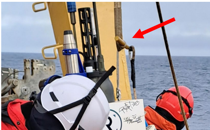
Detail of the axe allowing the release of the float for deployment
