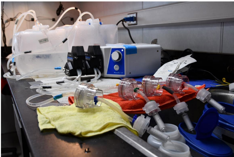
Figure 14-2: Sequential filtration performed in the laboratory shortly after sampling
