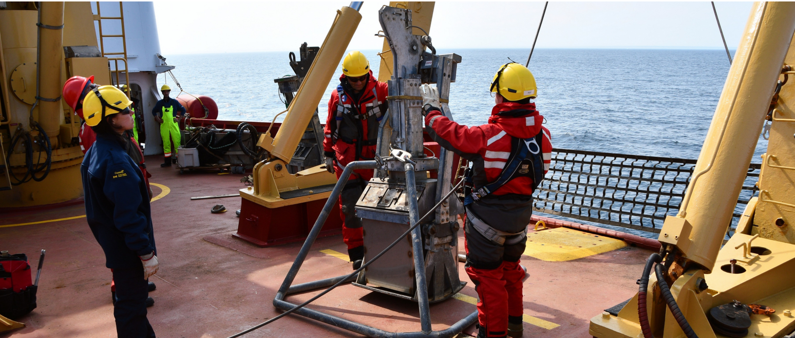
A box core being deployed from the CCGS Amundsen in order to collect sediment from the sea floor.
