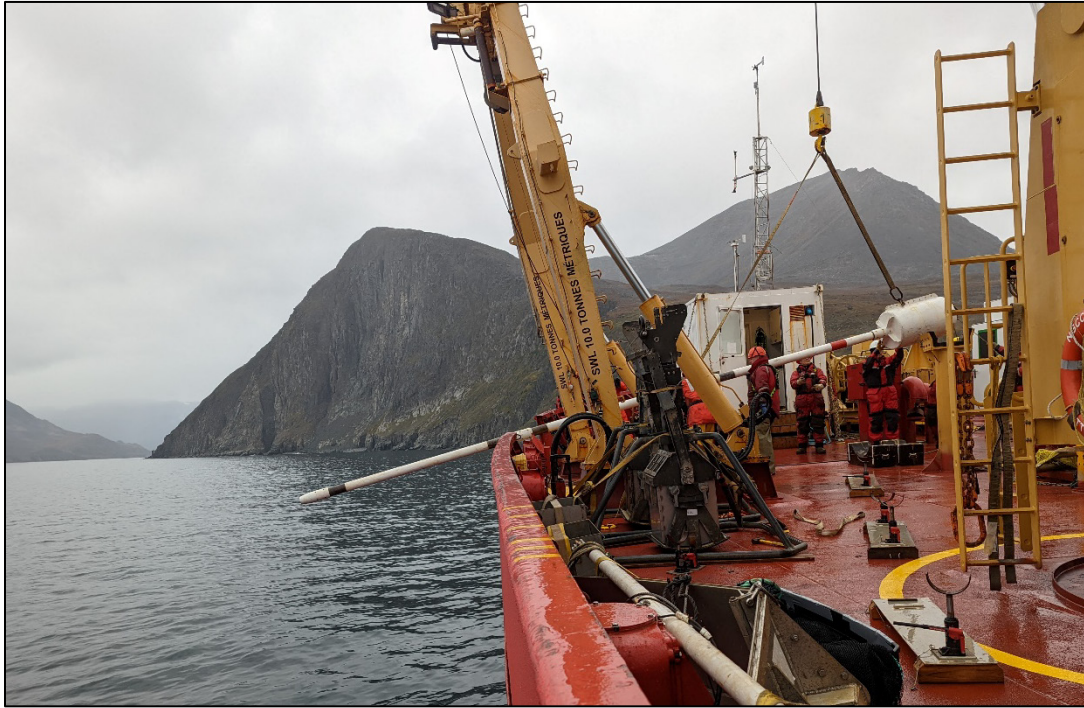
Figure 7-2: Gravity coring operations in Nachvak Fjord using the 9 m long piston corer
