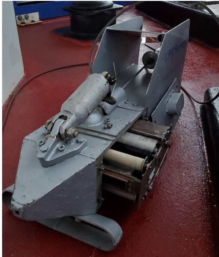
Figure 6-5. The continuous plankton recorder was used to sample the plankton community and microplastics in the upper water column (~5m) during leg 2. The photo also shows the internal sampling cassette being removed.
