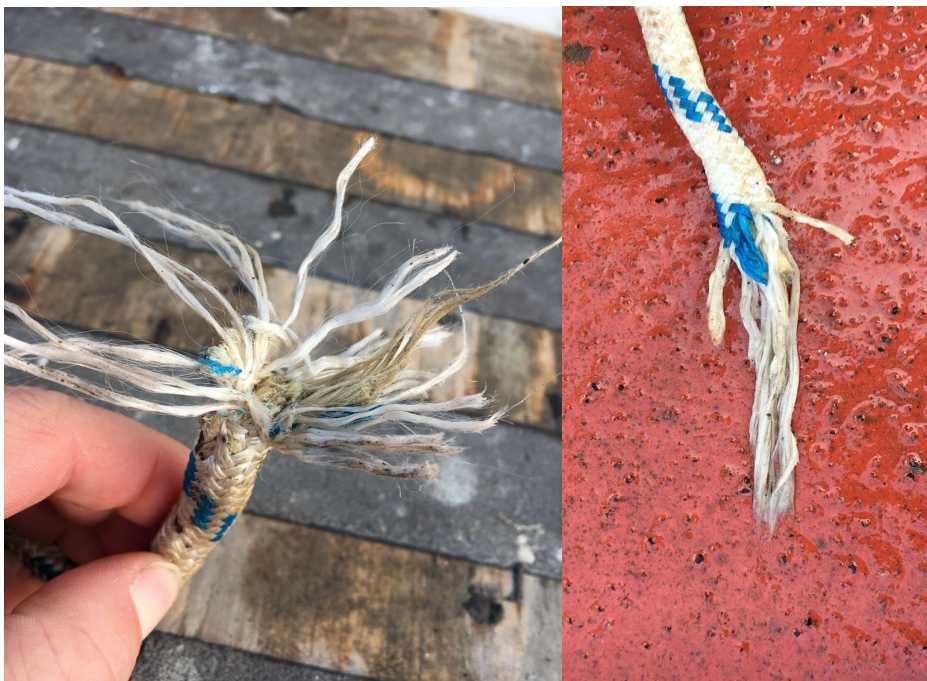
Figure 18-5. SagBank-21 mooring rope bow thruster cut point
