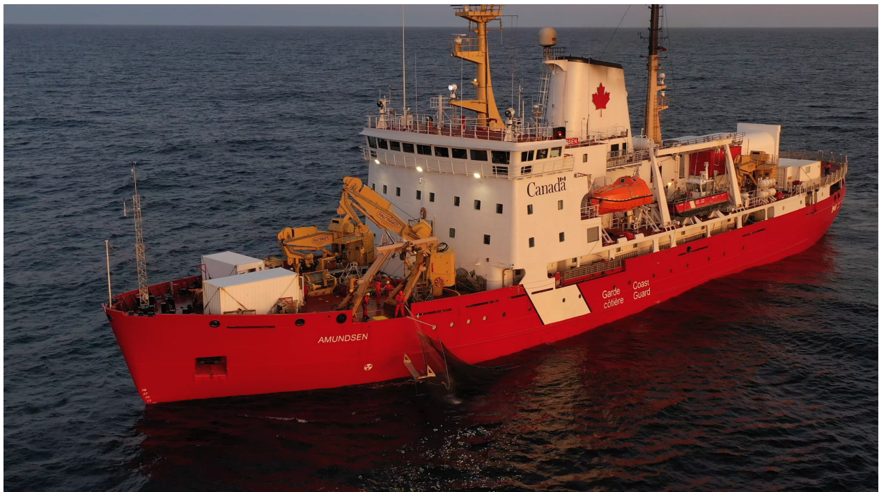
Figure 1-1: The CCGS Amundsen in the Labrador Sea during Leg 1. An Isaacs's Kidd midwater trawl (IKMT) is deployed with the A-Frame.
