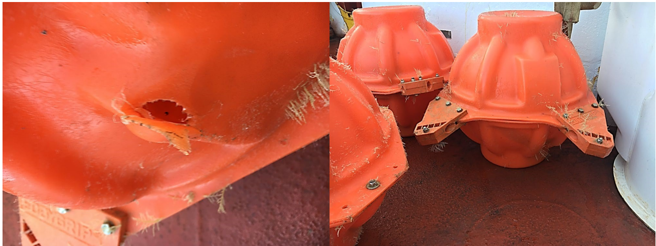
Figure 18-4. SagBank-21 glass sphere damage by bowthruster
