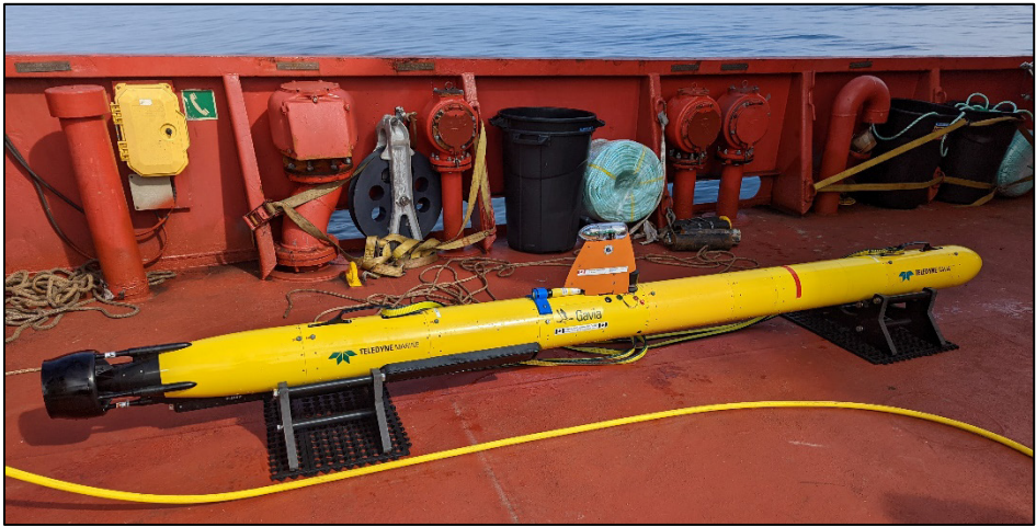
Figure 7-3: AUV used to collect high-resolution bathymetric data in Joey's Gully and Nachvak Fjord
