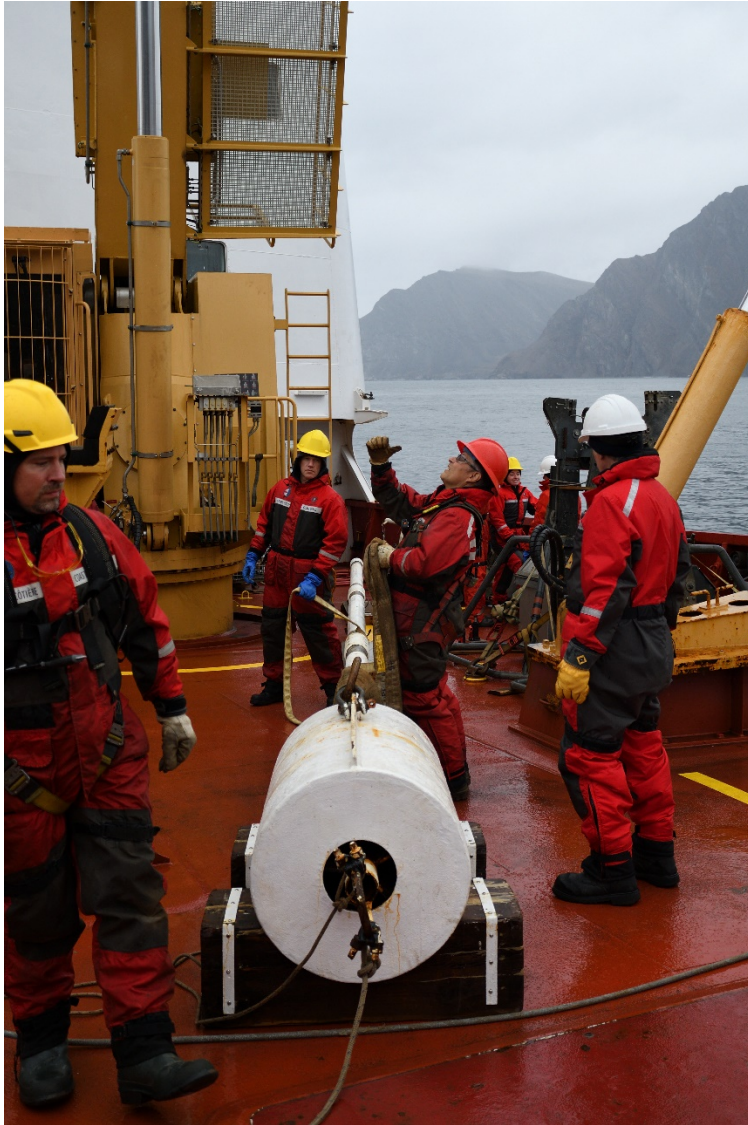
Figure 9-2: Gravity core being deployed.
