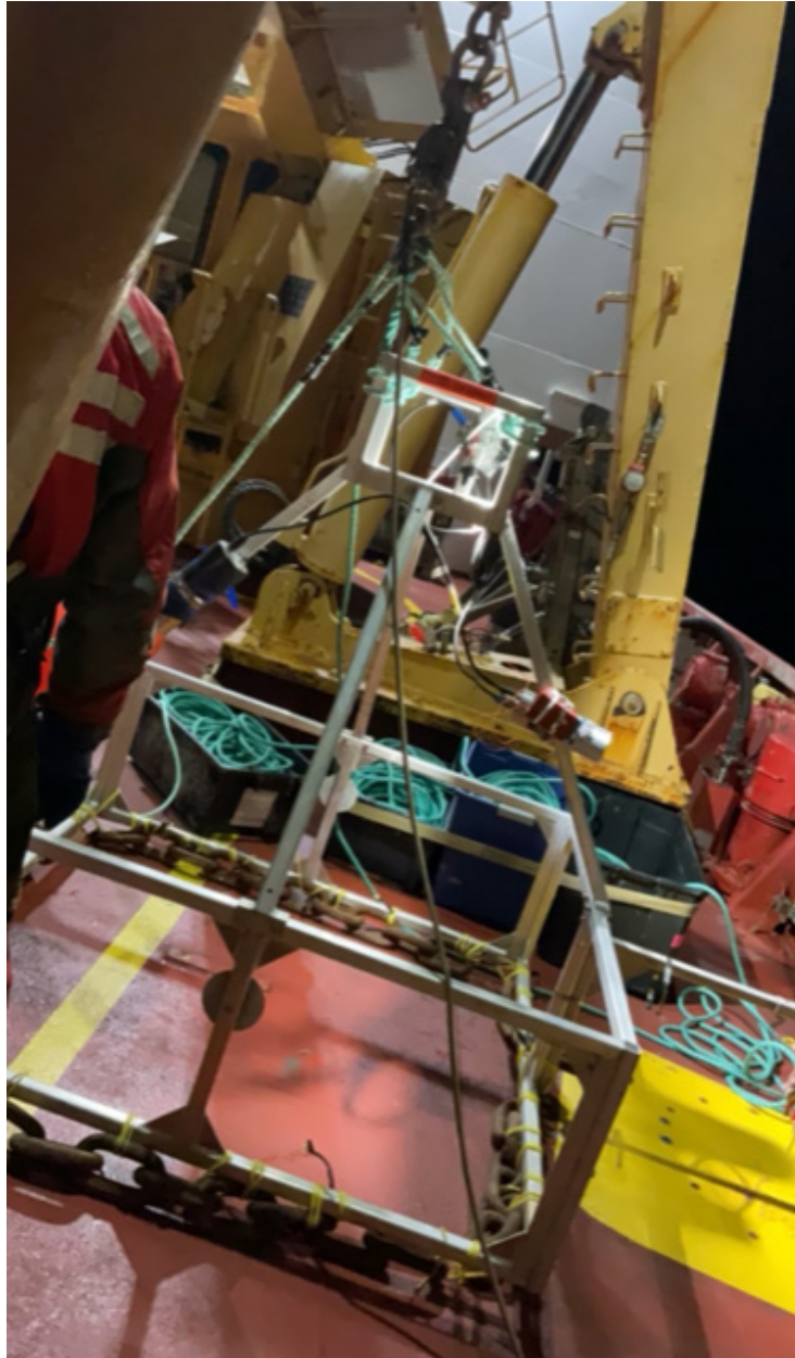
Figure 10-2: Baited camera equipped with both the Sony and 1Cam (mounted side by side near the bait arm). Chain was attached to the frame to stabilize it in the bottom and reduce drift, rope was coiled in figure 8 patterns in the boxes behind the frame. The 1Cam was connected to both the battery and the SubC light, attached on the top end of the frame.
