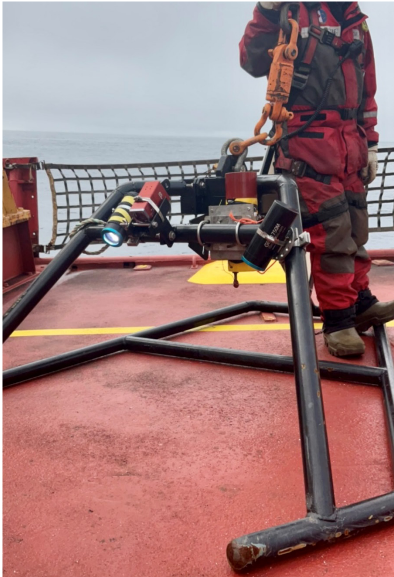
Figure 11-1: The drop camera system attached to a modified box-core frame utilized in Leg 1 of the 2022 Amundsen expedition.
