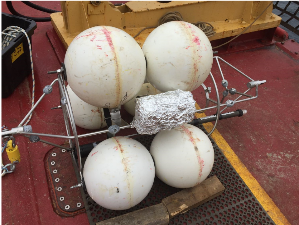
Figure 18-3. SPMD POPs trap ready for deployment on SagBank-21 (example image)
