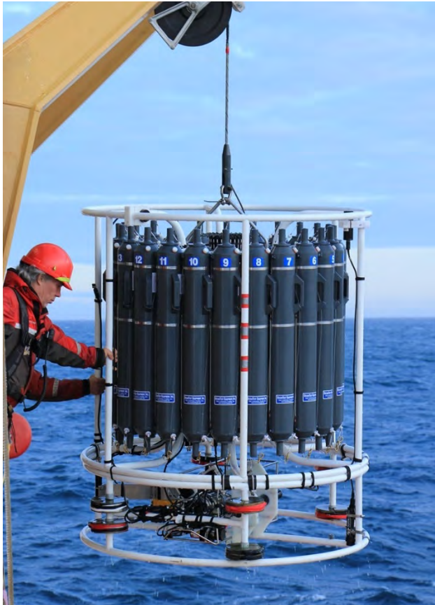
Figure 34-2: CTD rosette system being deployed by A frame from the starboard side of the ship
