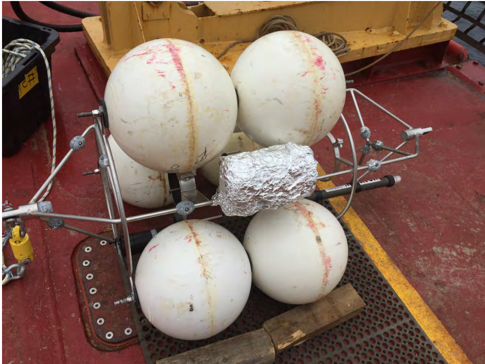
Figure 8-2: SPMD POPs trap ready for deployment on SagBank-21
