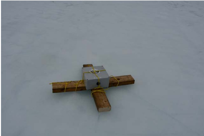
Figure 3-4: Replacement Cryologger beacon #4 with attached wooden frame, deployed August 23, 2021.
