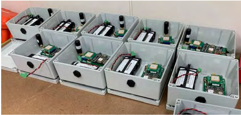
Figure 3-1: View of the interior of the Cryologger beacons deployed during the 2021 Amundsen Expedition Leg 3.
