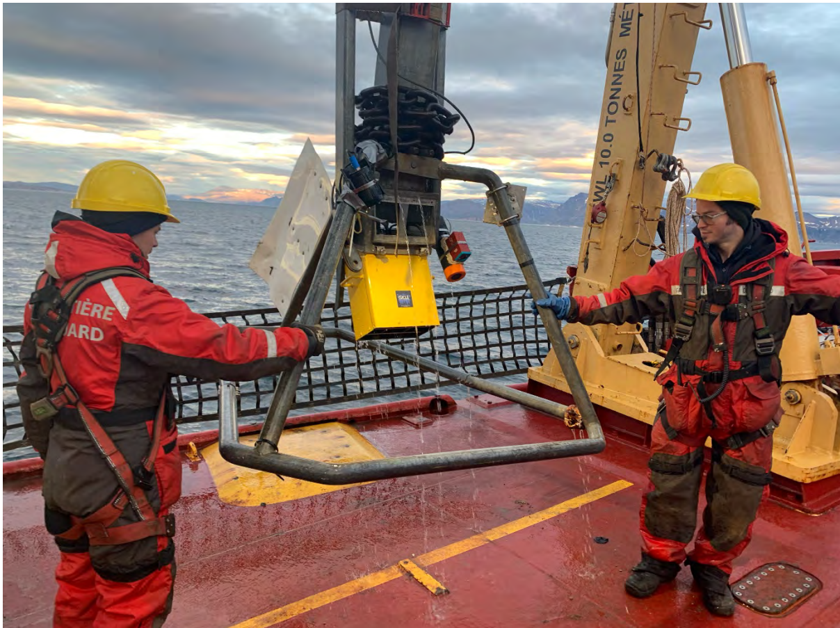
Figure 32-1: The drop camera system attached to a modified box core frame utilized in Leg 2 of the 2021 Amundsen Expedition
