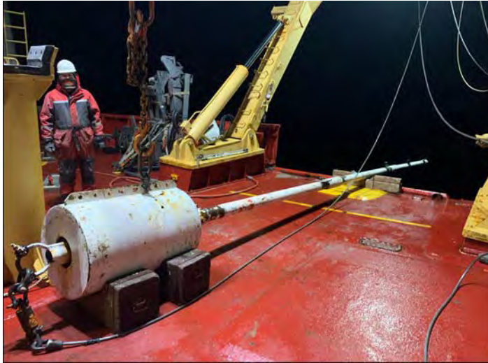
Figure 35-6: Giant gravity corer (9 m) on the fore-deck of the CCGS Amundsen awaiting deployment (@ M.-E. Rodriguez-Cuicas).
