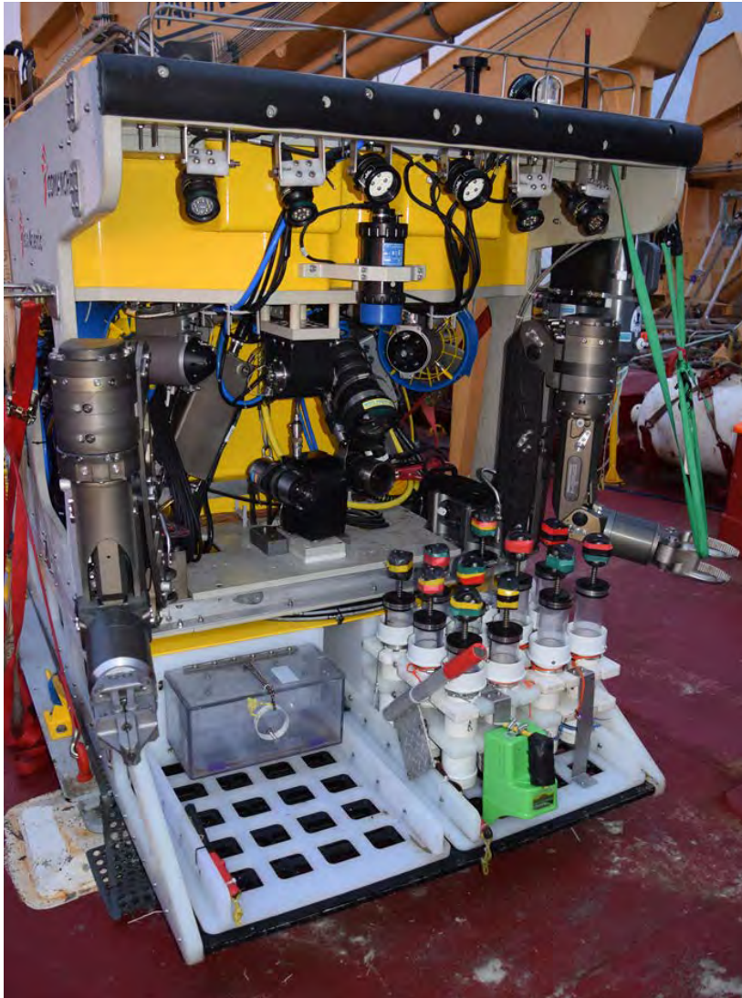
Figure 29-2: A) Comanche 38 ROV, fully loaded on the CCGS Amundsen foredeck before Dive 24 at Scott Inlet. Note two multifunction arms, porch for holding larger tools including 11 push cores in holsters, sampling skid, with lexan box and green sediment scoop for an additional method of sampling surface sediments. The sampling skid contains two hydraulically operated sample drawers, port and starboard, which can be opened independently. Mini-zeus camera is above, 1Alpha-Cam is below starboard, and additional pilot camera is blow port.
