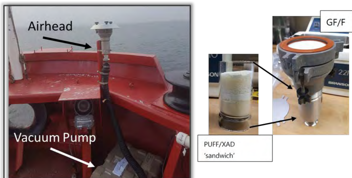
Figure 6-2: Air sampling setup and contents of air head; XAD glass column and glass fiber filter (GF/F).
