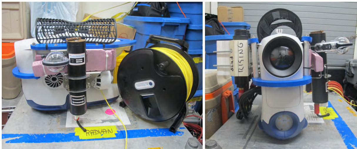
Figure 10-1: Remotely operated vehicle (ROV, Blueye Robotics) and attached sensors.
