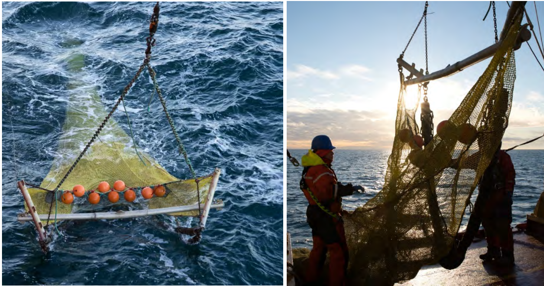
Figure 21-1: Beam trawl for sampling of benthic invertebrates
