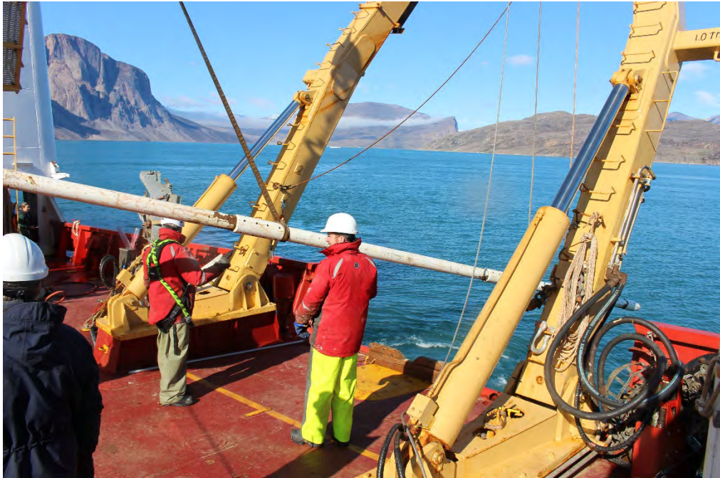
Figure 35-3: Deployment of the piston core
