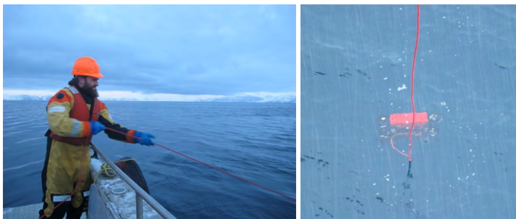
Figure 10-2: Deployment of the compact optical profiling system (C-OPS, Biospherical Instruments Inc.) from the barge.
