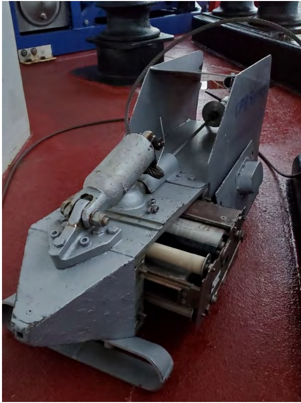
Figure 22-4: The continuous plankton recorder was used to sample the plankton community and microplastics in the upper water column (~5m) during leg 3. The photo also shows the internal sampling cassette being removed.
