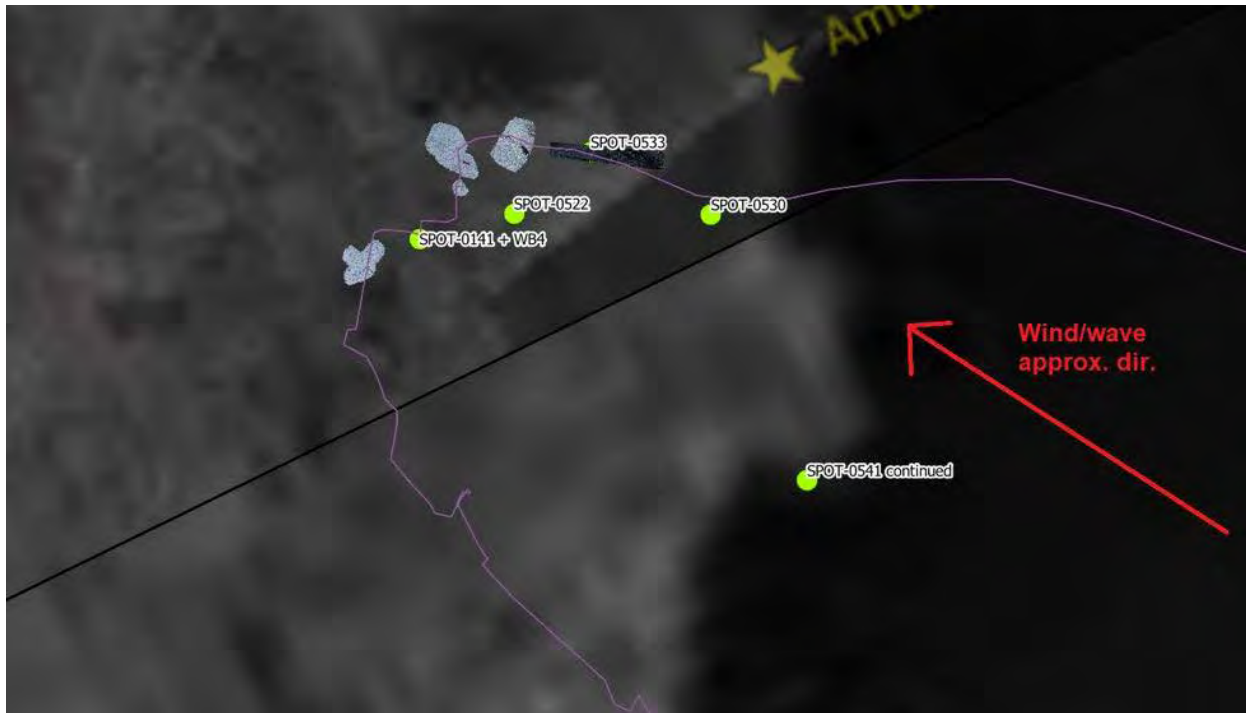
Figure 4-5: Geographical configuration of deployment DE330. A line of wave buoys was deployed from the outer MIZ extending approximately 7km into the MIZ. Note that the MIZ was highly dynamic and neither of the two SAR images in the background were taken at precisely the same time as the deployment or each other.
