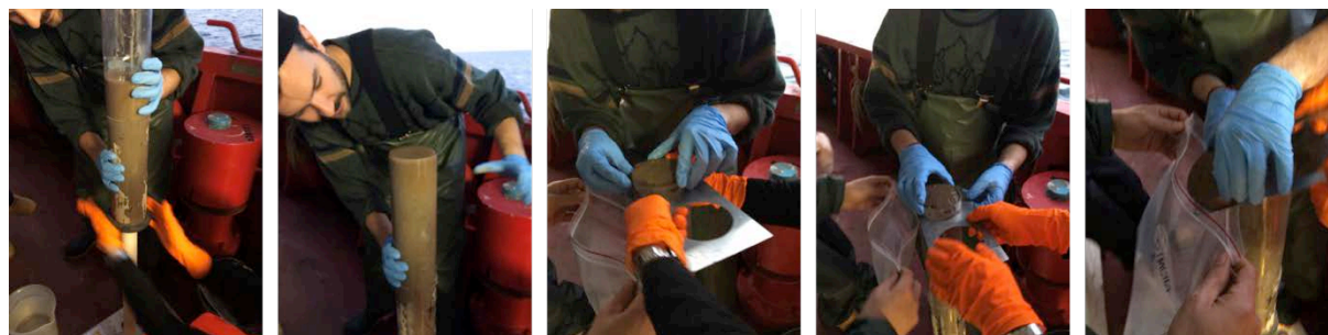
Figure 34-5: A sequence of images illustrating the slicing a sediment core from the MUC
