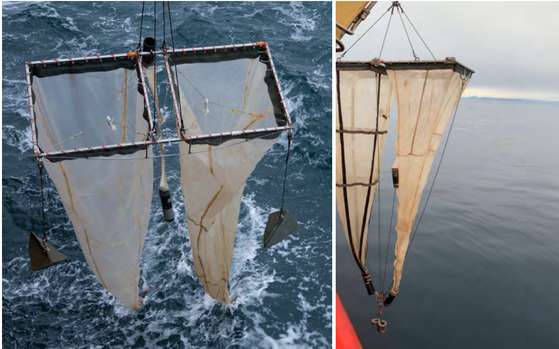
Figure 21-2: Oblique tow (Tucker; left) and vertical net (Monster; right) for sampling of zooplankton
